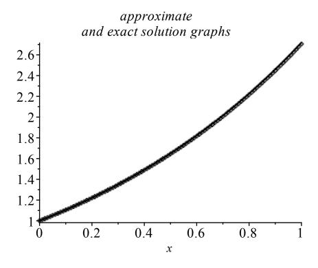
Exercise 3: For this very special initial value problem which has  $\exp(x)$  as the solution, set up Euler on the *x*-interval [0, 1], with *n* subdivisions, and step size  $h = \frac{1}{n}$ . Write down the resulting Euler estimate for  $\exp(1) = e$ . What is the limit of this estimate as  $n \to \infty$ ? You learned this special limit in Calculus!
