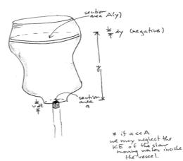
Experiment fun! I've brought a leaky nalgene canteen so we can test the Toricelli model. For a cylindrical tank of height h as below, the cross-sectional area A(y) is a constant A, so the Toricelli DE and IVP becomes
