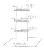
For the unforced (homogeneous) problem, the accelerations of the three massive floors (the top one is the roof) above ground and of mass m, are given by
