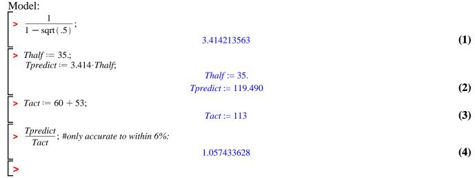
Notice that the experiment is close, but doesn't exactly match the prediction. Aside from experimental inaccuracies, can you think of places in which the model itself is inexact (there are several)?
