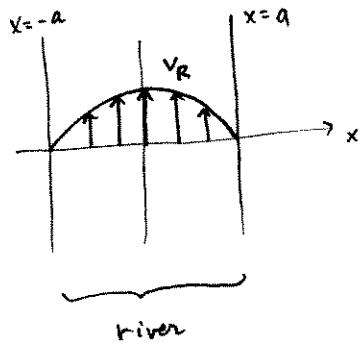
$$v_R = v_0 \left(1 - \frac{x^2}{a^2}\right) \quad \text{is velocity profile of river water}$$
