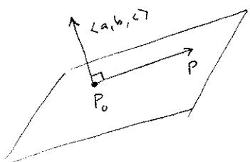
geometrically describes a plane through  $P_0$  with normal ( $\perp$ ) vector  $\langle a, b, c \rangle$ !i.e. the plane is the set of
