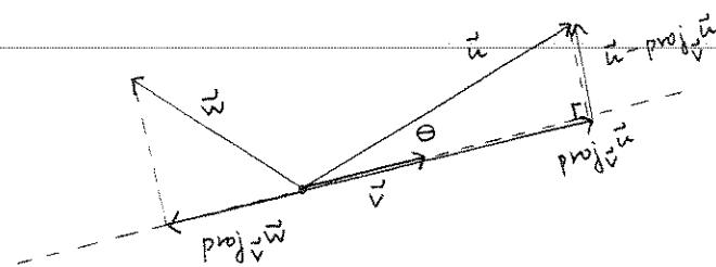
$$\text{proj}_{\vec{v}} \vec{u} = \underbrace{|\vec{u}| \cos \theta}_{\text{dist}} \underbrace{\frac{\vec{v}}{|\vec{v}|}}_{\text{unit vect in } \vec{v} \text{ dir}}$$
