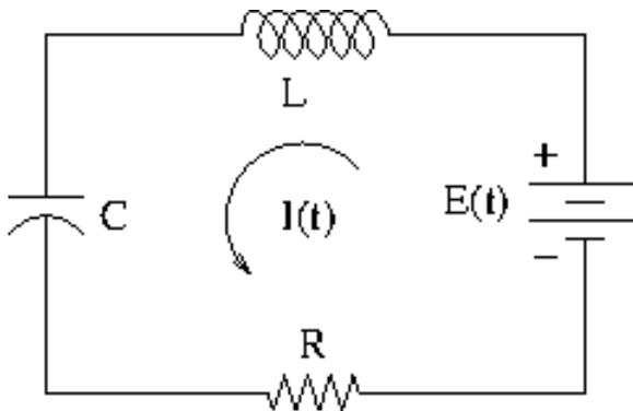
**The Problem.** Suppose  $E = 100 \sin(20t)$ ,  $L = 5$  H,  $R = 250 \Omega$  and  $C = 0.002$  F. The model for the charge  $Q(t)$  is  $LQ'' + RQ' + \frac{1}{C}Q = E(t)$ .
