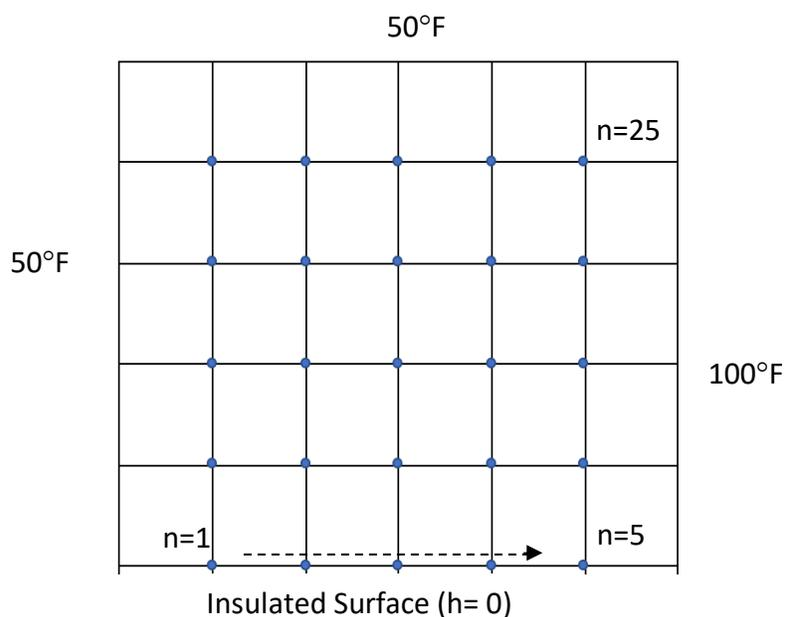
Since there is insulation, there is no heat transfer along the bottom surface, so the temperature increases significantly along the bottom of the plate. In the case of constant temperature, the temperature had a less significant gradient along the bottom of the plate.
