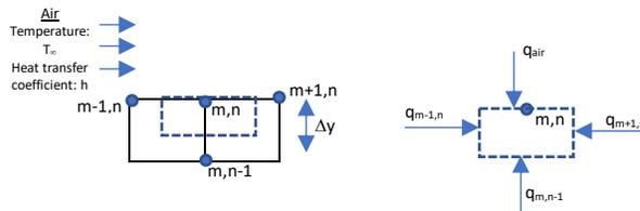
Using the same principles of energy balance and heat flux, the equation for the temperature at node (m,n) can be derived.
