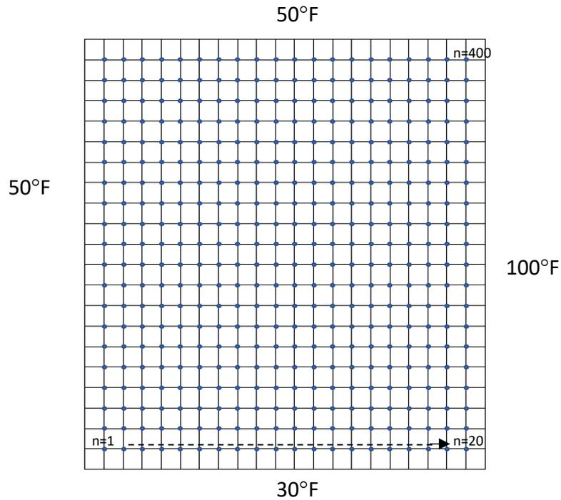
Using the same process as above, the matrix  $[A]$  of equations at each node can be obtained. The matrix is size  $400 \times 400$ , so the details are omitted. Once the vector of temperatures at each node is solved for, a contour plot of the temperature distribution can be created again.
