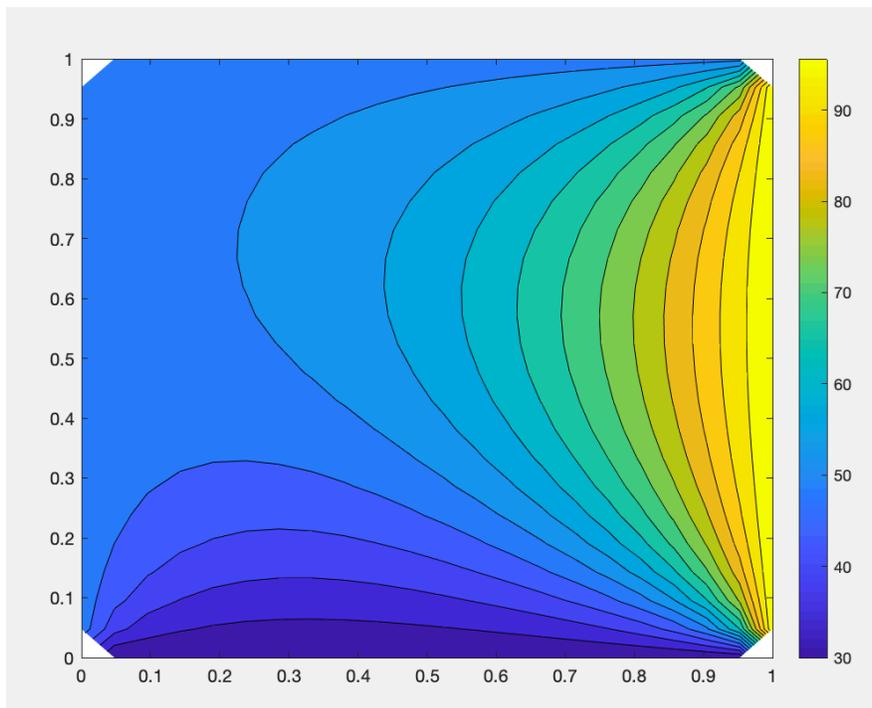
For the same boundary conditions on a heated plate, as the number of nodes increases, the discontinuities in the temperature distribution across nodes transition to a more continuous distribution. To achieve the most accurate approximation, increase the number of nodes until there are an infinite number of nodes within the plate.
