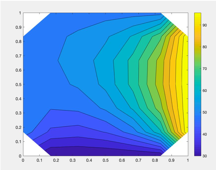
Now, the number of nodes along each row was increased from  $n = 5$  to  $n=20$  to show how the temperature distribution changes, with the same boundary conditions
