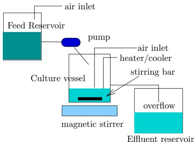
**Figure 8. Laboratory Chemostat.**
