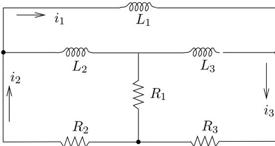
**Figure 17. An electrical network.** There are three resistors  $R_1, R_2, R_3$  and three inductors  $L_1, L_2, L_3$ . The currents  $i_1, i_2, i_3$  are defined between nodes (black dots).
