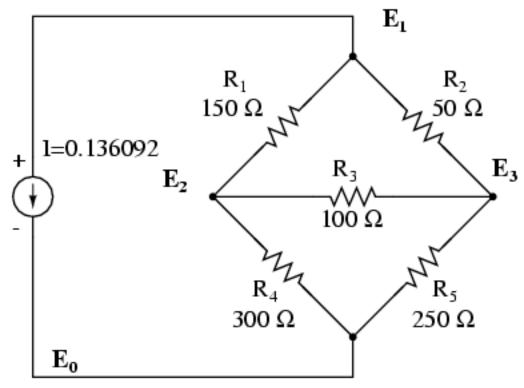
Once the matrices are set up, we'll find the Circuit current in each network using simple Row Reduction in Maple.
