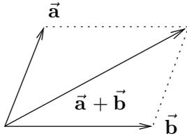
**Figure 14. The parallelogram rule.**
