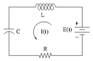
**The Problem**. Suppose  $E = 100 \sin(20t)$ , L = 5 H,  $R = 250 \Omega$  and C = 0.002 F. The model for the charge Q(t) is  $LQ'' + RQ' + \frac{1}{C}Q = E(t)$ .
