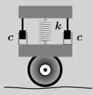
Figure 6. A trailer strut with dampers on a washboard road
