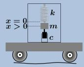
**Figure** 2. A spring-mass system with damper in a box transported in an auto trunk along a washboard road.
