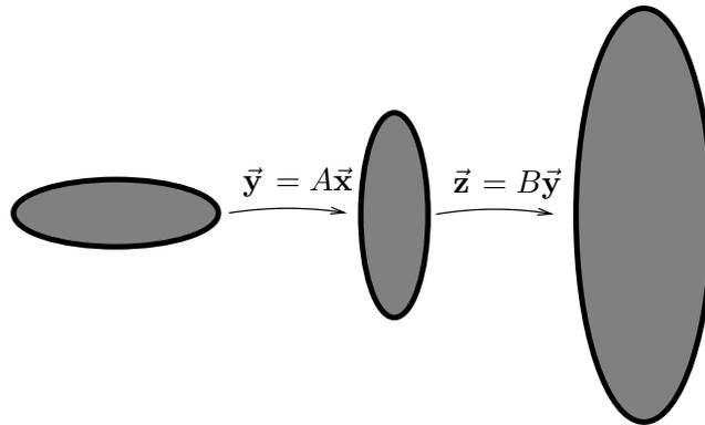
**Figure 9.** An ellipse is mapped into a rotated and re-scaled ellipse. The rotation is  $\vec{y} = A\vec{x}$ , which is followed by re-scaling  $\vec{z} = B\vec{y}$ . The composite geometric transformation is  $\vec{z} = BA\vec{x}$ , which maps the ellipse into a rotated and re-scaled ellipse.
