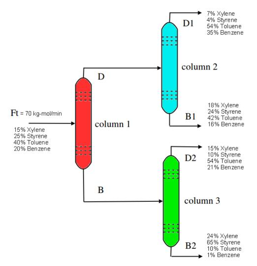
**Balance Equations**. The four Xylene separations imply balance equation 0.07D1 + 0.18B1 + 0.15D2 + 0.24B2 = 0.15(70) kg-mol, based on 1 min of operation. There are 3 other similar equations, for styrene, toluene and benzene. Multiply by 100 to produce the balance equations
