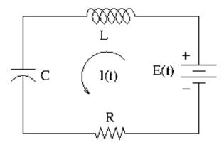
**The Problem.** Suppose  $E = \sin(40t)$ , L = 1 H,  $R = 50 \Omega$  and C = 0.01 F. The model for the charge Q(t) is  $LQ'' + RQ' + \frac{1}{C}Q = E(t)$ .
