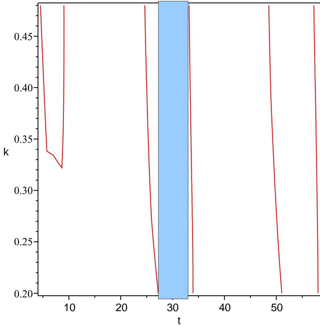
The blue rectangle replaces the region R between the two red curves. Inequalities describe the rectangle:  $27 < t < 33$ ,  $0.2 < k < 0.5$ . Meaning: for 27 to 33 hours, the temp surface is below the plane  $z=30F$ , hence freezing occurs, for all insulation constants  $k$  from 0.2 to 0.5.
