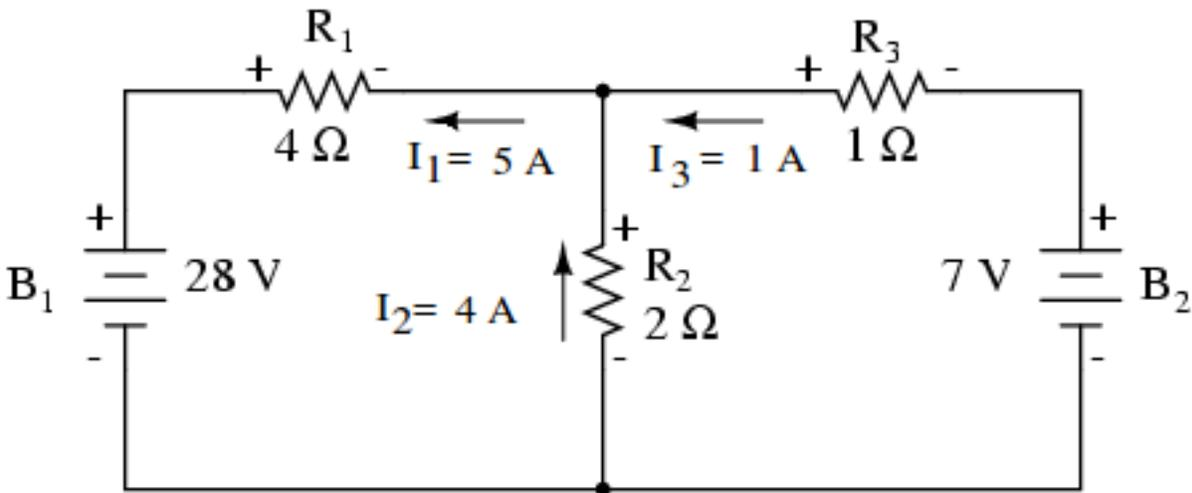
The **Branch Current Method** can be used to find a  $3 \times 3$  linear system for the **branch currents**  $I_1, I_2, I_3$ .
