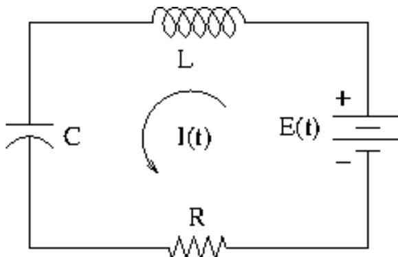
**The Problem.** Suppose  $E = \sin(40t)$ ,  $L = 1$  H,  $R = 50 \Omega$  and  $C = 0.01$  F. The model for the charge  $Q(t)$  is  $LQ'' + RQ' + \frac{1}{C}Q = E(t)$ .
