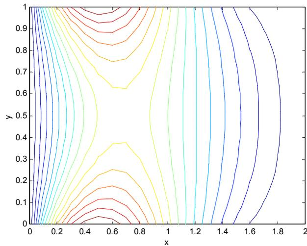
Suppose now, that the boundary conditions are such that  $f_1(x) = 3 f(x) = 3 x (L - x)^3$  and  $g_1(x) = 5 g(x) = 5 x^3 (L - x)$ . Since we already have the solutions corresponding to  $f(x)$  and  $g(x)$ , we can obtain the solution to the problem with the new set of boundary conditions by constructing the following solution  $u(x, y) = 3 u_1(x, y) + 5 u_2(x, y)$ :
