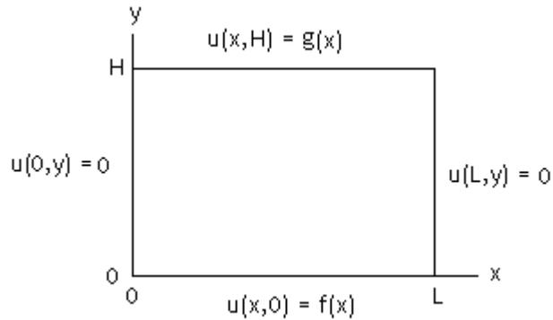
We use for the solution  $f(x) = x(L-x)^3$ , and  $g(x) = x^3(L-x)$ . Thus, we can simply add the results from cases 1 and 2, namely,  $uu1+uu2$ , and plot a surface plot of these results:
