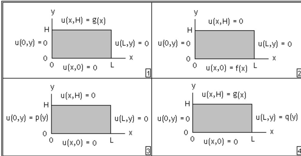
[12]. Referring to the figure of problem [12], solve case [4] of Laplace's equation in the rectangular domain  $L = 2$ ,  $H = 1$ , if  $q(y) = (y/H)^2(1-y/H)$ . Produce a surface plot as well as a contour plot of the results.
