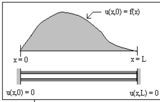
We will try to find a solution by the method of separation of variables. This method assumes that the solution,  $u(x,t)$ , can be expressed as the product of two functions,  $X(x)$  and  $T(t)$ :
