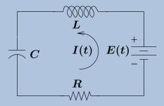
Figure 1. An LRC Circuit.
