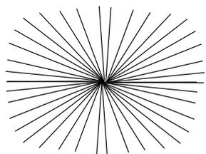
Figure 12. Proper node
