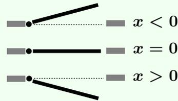
**Figure 5.** Top view of a cafe door, showing the three possible door positions. Figure 5 shows that, for modeling purposes, the cafe door can be reduced to a torsional pendulum with viscous damping. This results in the **cafe door** equation
