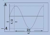
Figure 1. Simple harmonic oscillation  $x(t) = A \cos(\omega t - \alpha)$ , showing the period  $2\pi/\omega$ , the phase shift  $\alpha/\omega$  and the amplitude A.
