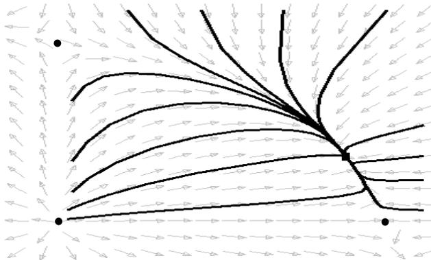
**Figure 10. Phase Portrait for Trout System (6).** Shown are typical solution curves and a direction field. Equilibrium  $(80, 20)$  is asymptotically stable (a square). Equilibria  $(0, 60)$ ,  $(90, 0)$ ,  $(0, 60)$  are unstable (circles).
