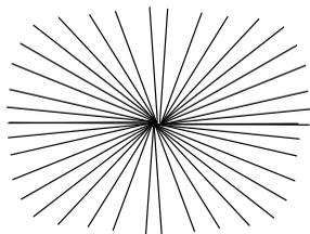
Figure 14. Proper node
