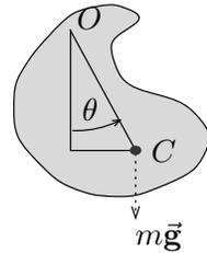
Figure 6. The physical pendulum
