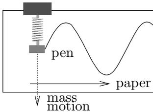
**Figure 4.** A moving paper chart records the vertical motion of a mass on a spring by means of an attached pen.
