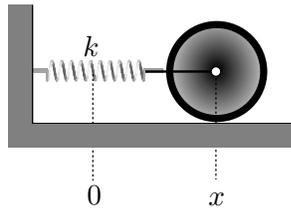
**Figure 10.** A rolling wheel attached to a spring.
