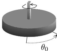
**Figure 8.** The torsional pendulum, a model for a balance wheel in a watch. The wheel rotates angle  $\theta_0$  about the vertical axis, which acts as a spring, exerting torque  $I$  against the rotation.
