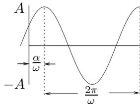
**Figure 3.** Simple harmonic oscillation  $x(t) = A \cos(\omega t - \alpha)$ , showing the period  $2\pi/\omega$ , the phase shift  $\alpha/\omega$  and the amplitude  $A$ .
