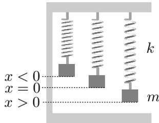
**Figure 2.** An undamped spring-mass system, showing compression, equilibrium and elongation of the spring with corresponding positions of the mass  $m$ .
