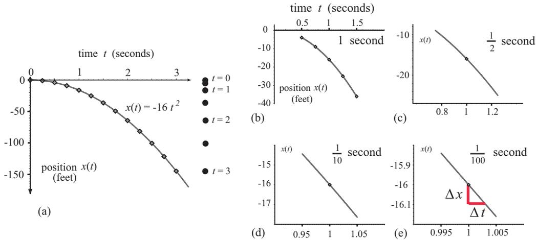
Figure 1.11: (a) Data on the position of a falling pebble at time intervals of 0.25 seconds. The function  $x(t) = -16t^2$  gives the position for any time  $t$ , neglecting air friction. (b)–(e) Zooming in on the graph of  $x(t)$  around  $t = 1$  shows that  $x(t)$  looks more and more linear when viewed on smaller and smaller time scales, like uniform motion in Figure 1.10.
