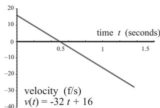
Figure 1.13: The instantaneous velocity of a ball thrown upward with an initial velocity of 16 f/s. The maximum height occurs at  $t = \frac{1}{2}$  when the velocity is 0.
