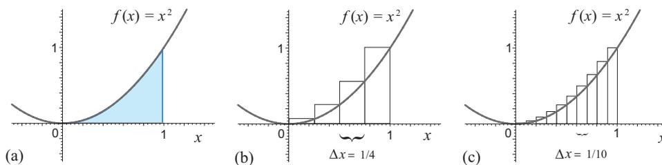
Figure 1.16: The area under the graph of the parabola  $f(x) = x^2$  over  $[0, 1]$  in (a) can be found from the antiderivative  $F(x) = x^3/3 + C$  of  $f(x)$ . Later, we'll look more closely at how this method is related to summing the areas of the boxes in (b) and (c).
