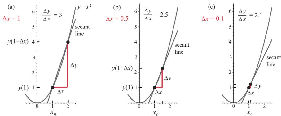
Figure 1.7: The secant line contains the two points on the graph of  $y(x) = x^2$  at  $x = x_0$  and  $x = x_0 + \Delta x$ , and *approximates* the tangent line at  $x = x_0$ . As  $\Delta x$  gets smaller, the approximation gets better, and the secant converges to the tangent as  $\Delta x \rightarrow 0$ .
