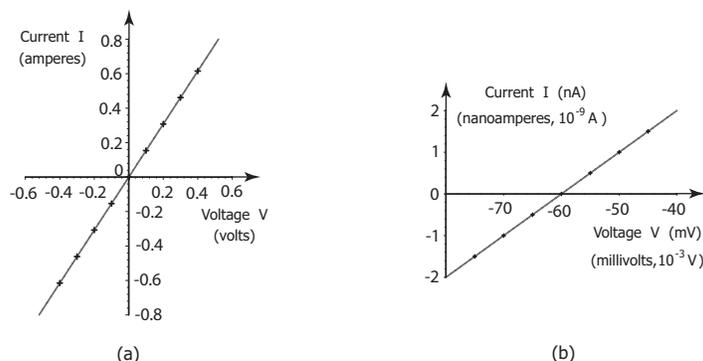
Figure 1.14: In (a), current *vs.* voltage data for a 100 foot copper wire exhibits Ohmic, or linear behavior [7]. Reversing the potential difference between the ends of the wire reverses the current direction. In (b) current *vs.* voltage data for a neuron is plotted.
