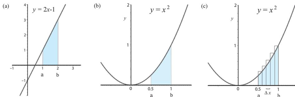
Figure 1.5: (a) The shaded region under the graph of the function  $y(x) = 2x - 1$  on  $[a, b]$  is a trapezoid with base width  $w = b - a$  and heights  $h_1 = y(a)$  and  $h_2 = y(b)$ . Its area is  $w \cdot (h_1 + h_2)/2 = 1 \cdot (1 + 3)/2 = 2$ . (b) The shaded region under the parabolic graph of  $y(x) = x^2$  on  $[\frac{1}{2}, 1]$  is *not* a shape whose area we know from basic geometry. (c) The area of the shaded region can be approximated by summing up the areas of the rectangles.
