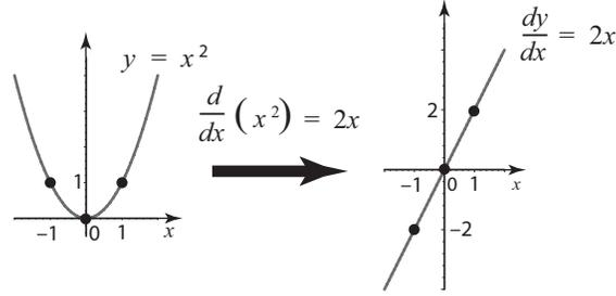
Figure 1.8: The derivative of  $y(x) = x^2$  is a new function  $dy/dx = 2x$  whose value at  $x_0$  is the slope of the tangent line at  $x = x_0$ . For example,  $\frac{dy}{dx}(-1) = -2$  and  $\frac{dy}{dx}(0) = 0$ .
