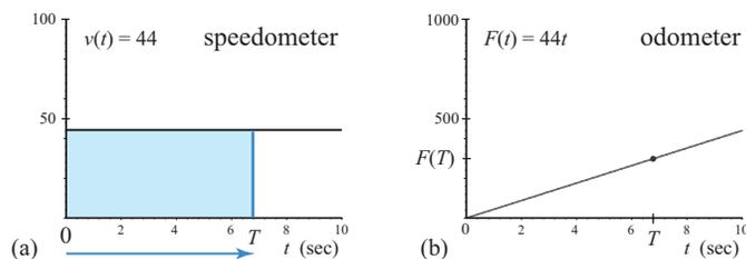
Figure 1.4: The odometer value  $F(T)$  in (b) after  $T$  seconds is the area of the shaded region under the graph of the speedometer function  $v(t)$  in (a) over the interval  $[0, T]$ .
