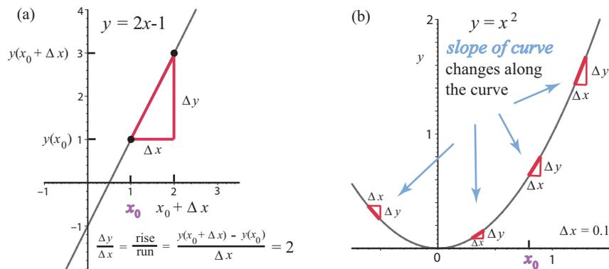
Figure 1.3: (a) The rate of change of  $y(x) = 2x - 1$  with respect to  $x$  is 2, the slope of the line. (b) The nonlinear function  $y(x) = x^2$  has a parabolic graph. The rate of change of  $y$  with respect to  $x$  at a point  $x = x_0$  is the *slope of the curve*, or the steepness there.
