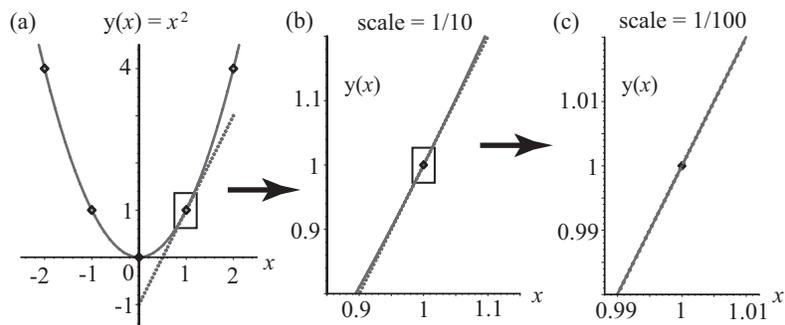
Figure 1.6: Zooming in on the graph of  $y(x) = x^2$  around  $x_0 = 1$ . In (a) the dotted line is tangent to the graph at  $x_0 = 1$ , intersecting only at the point  $(1, 1)$ . The slope of the curve at  $x_0 = 1$  is the slope of this tangent line. On smaller and smaller scales, as in (b) and (c), the tangent line becomes practically indistinguishable from the curve.
