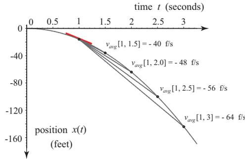
Figure 1.12: The average velocity over each time interval is the slope of the *secant line*. As the interval becomes smaller and smaller, the secant lines approach the red tangent line.
