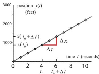
Figure 1.10: High-speed train in uniform motion. Displayed on the right is data on its position  $x$  in feet *vs.* time  $t$  in seconds, taken at 1 second intervals.
