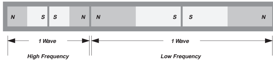
Figure 9.16: Recorded information on magnetic tape.
