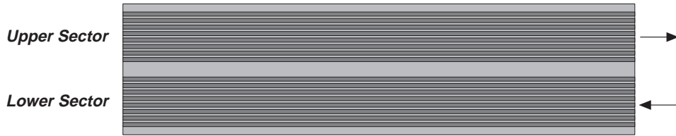
Figure 11.8: Track pattern in DCC tape.
