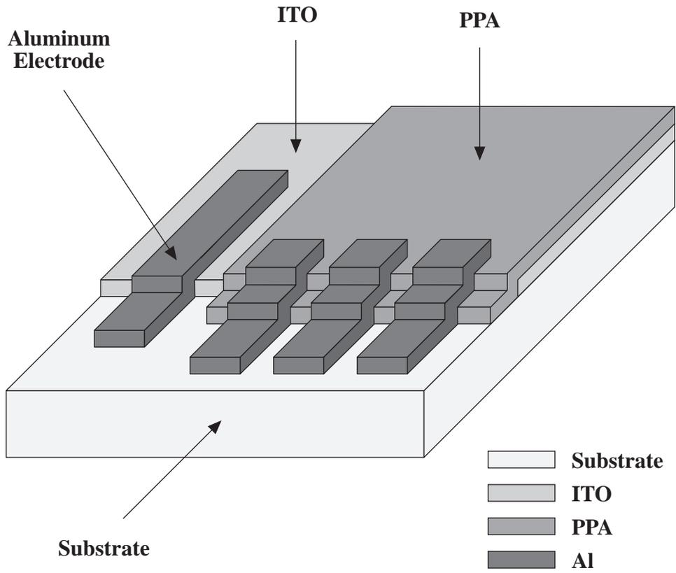
Figure 7.1: Al/PPA/ITO Diode Device Construction (not to scale).
