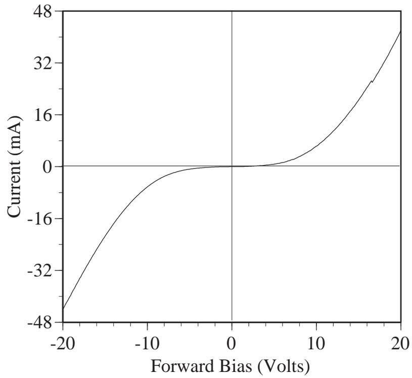
Figure 7.2: I-V Characteristic of symmetric Al/PPA/ITO Diode.
