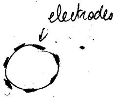
find conductivity inside  $\Omega$  that better fits electrical measurements at boundary
