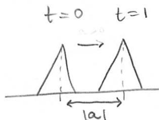
Solution is a "pulse" traveling at speed  $a$ . Sign of  $a$  gives direction of propagation.
