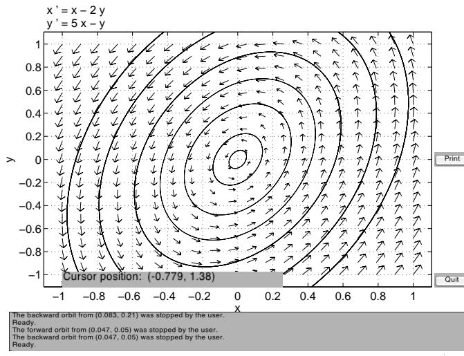
(6.2.12) The system is of the form  $\underline{x}' = A \underline{x} + \underline{b}$
