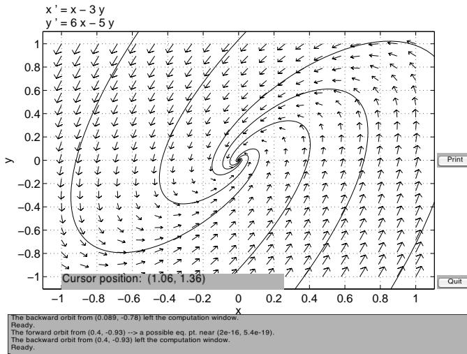
6.2.10  $\underline{x}' = A \underline{x}$  with  $A = \begin{bmatrix} 1 & -2 \\ 5 & -1 \end{bmatrix}$ ;  $\rho(\lambda) = (1-\lambda)(-1-\lambda) + 10 = \lambda^2 + 9 = (\lambda - 3i)(\lambda + 3i)$
