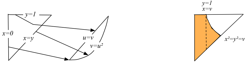
Figure 25.1. Domains for pdfs in Example 25.4. Left: domain transformation. Right: integration area for CDF calculation.
