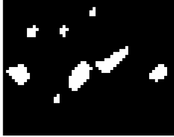
Figure 5: The Betti numbers of a binary image from one of 2D slices of columnar ice. Betti number of black pixels is \beta_0 = 1 and \beta_1 = 8 . On the other hand, Betti number of white pixels is \beta_0 = 8 and \beta_1 = 0 .
