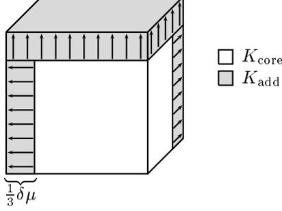
FIGURE 1. Replacing orthogonal strips in the differential scheme. The arrows in the added material indicate the direction of the conductivity eigenvalue  $k_n$ .
