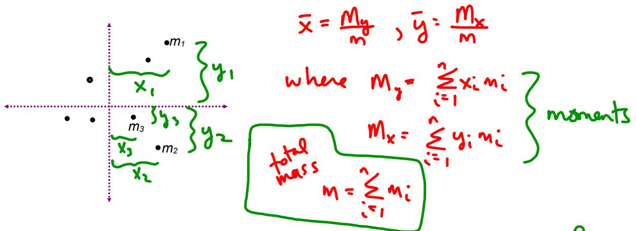
note:  $M_y$  is the "x moment" measured from the y-axis
