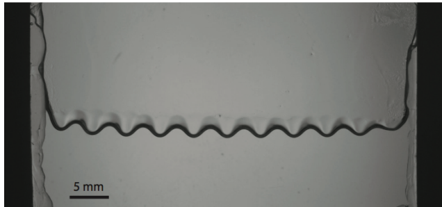
Figure 5: Square cell half-filled with ethanol 70% undergoing vertical oscillation, above the instability threshold, at f = 85 Hz. (Provided by Lionel Vincent)
