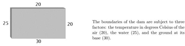
An analysis of the heat transfer from the three sources will be done from the equilibrium temperature, which is found by the Mean Value Property below.
