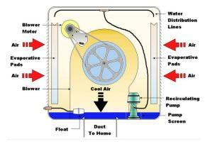
An evaporative cooler, used in low-humidity regions of the United States instead of refrigerated air conditioning.
