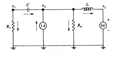
Figure 3: A simple RLC circuit
