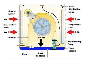
An evaporative cooler, used in low-humidity regions of the United States instead of refrigerated air conditioning.
