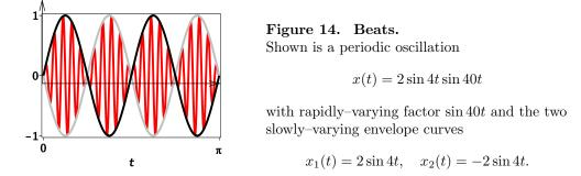
A key example is piano tuning. A tuning fork is struck, then the piano string is tuned until the beats are not heard. The number of beats per second (unit Hz) is approximately the frequency difference between the two sources, e.g., two tuning forks of frequencies 440 Hz and 437 Hz would produce 3 beats per second.
