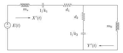
Figure 31. Dynamic shock absorber simulator circuit (2009)
