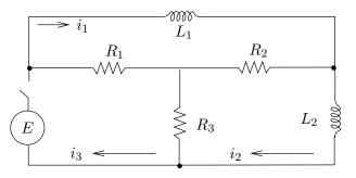
Figure 18. An electrical network. There are three resistors  $R_1$ ,  $R_2$ ,  $R_3$ , two inductors  $L_1$ ,  $L_2$  and a battery E. The currents  $i_1$ ,  $i_2$ ,  $i_3$  are defined between nodes (black dots).
