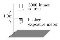
Figure 3. Jeweler's bench experiment. The exposure meter measures light intensity at the beaker's base.
