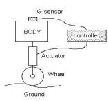
Figure 29. Active Suspension Components.
