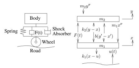
Figure 32. One wheel suspension with spring, shock absorber and regulator F(t). Variables and forces are defined in the force diagram on the right. All units MKS.
