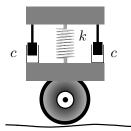
Figure 23. A trailer strut with dampers on a washboard road
