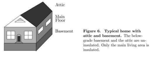
It is usual to surround the main living area with insulation, but the attic area has walls and ceiling without insulation. The walls and floor in the basement are insulated by earth. The basement ceiling is insulated by air space in the joists, a layer of flooring on the main floor and a layer of drywall in the basement. We will analyze the changing temperatures in the three levels using Newton's cooling law and the variables
