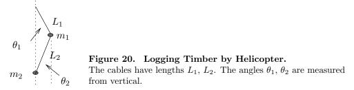
The lengths  $L_1$ ,  $L_2$  are adjusted on each trip for the length of the trees, so that the trees do not collide in flight with each other nor with the helicopter. Sometimes, three or more smaller trees are bundled together in a package, which is treated here as identical to a single, very thick tree hanging on the cable.
