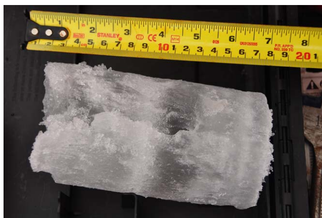
Figure 16. Image of a core section showing centimeter+ scale pore space common in deteriorating ice.
