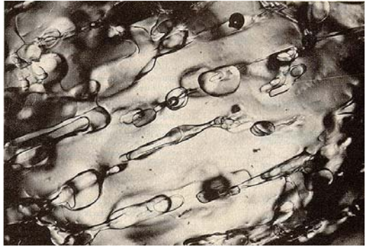
Figure 5. Sub-millimeter scale brine inclusions in sea ice. (W. Weeks and A. Assur)
